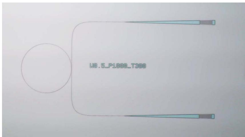
Figure 1. Microscope capture showing resolved Nitride ring resonator waveguide design with grating coupler pitch of 1000nm.
