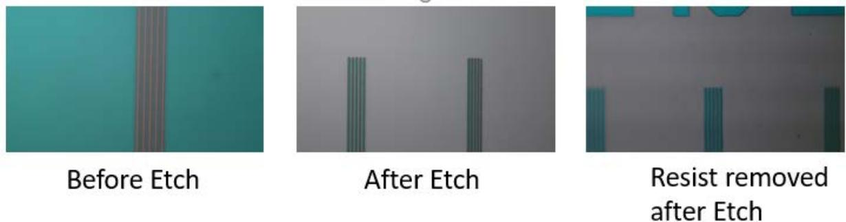
Figure 1. 1.0um line/space imaging before etch and after etch and after resist removal.
