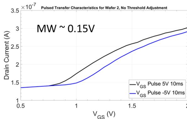
Figure 1. Transfer Characteristics of an n-channel FeFET shows Memory Window of 150mV.
