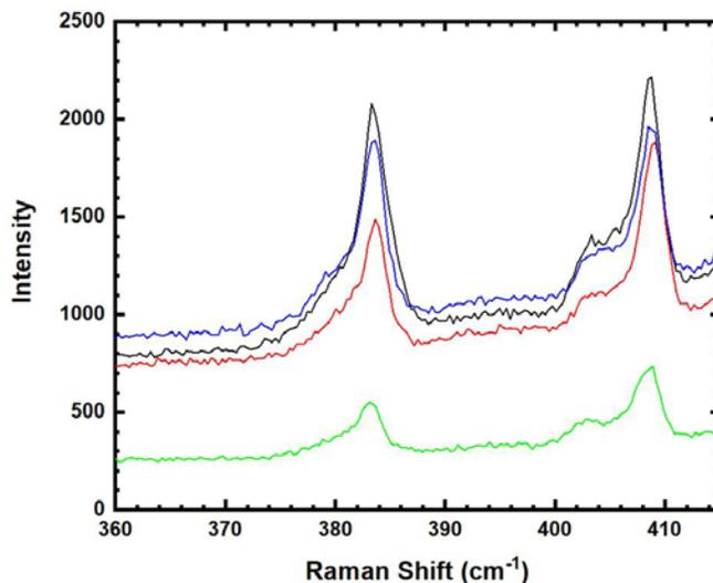
**Figure 1.** This figure demonstrates the different Raman Shift profile inspected on different atomic layers of exfoliated MoS<sub>2</sub>
