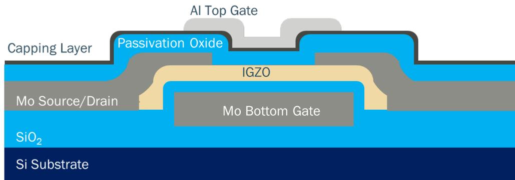
Figure 1. Cross section of an IGZO TFT.
