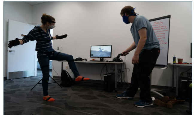
Fig. 2. Recording Motion Capture data with a virtual camera using the Perception Neuron mocap suit and the Unreal engine
