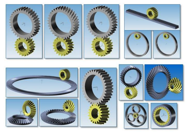
Some of the latest developments are the generation of offset face gear drives and the generation of doubleenveloping (globoidal) worm gear drives.
