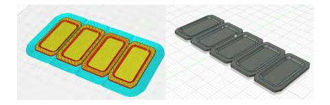
The second design iteration modified the larger sections to demonstrate different printing features, while smaller test 'fins' were included for material testing and designed to detach.
