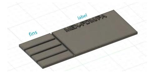
The final measurements of this design are L x W x H 91.5 mm x 36.5 mm x 2.5 mm. With additional text, the total height is 3.5 mm. The gap between the 'fins' is 1.5 mm, and the gap height is 0.5 mm. The overall height and the gap height were modified as needed during printing for specific technology types.
