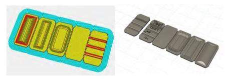
The final design (pictured below) maintained these detachable 'fins', but the larger section was simplified and included a label printed onto the sample surface.
