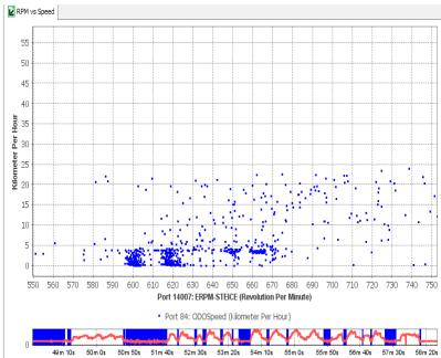
Example screens from the MGUI tool showing collected data from a vehicle application
