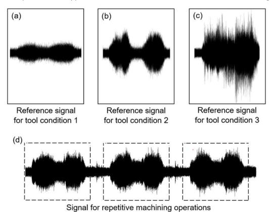
Reference signals (a, b, and c) are generated by cutting tools with different conditions during the calibration procedure. By comparing the signal for actual repetitive machining operations (d) with the signals for different tool conditions (a, b, and c), it can be realized that the actual tool condition should be between tool conditions 2 and 3 and closer to the condition 2.
