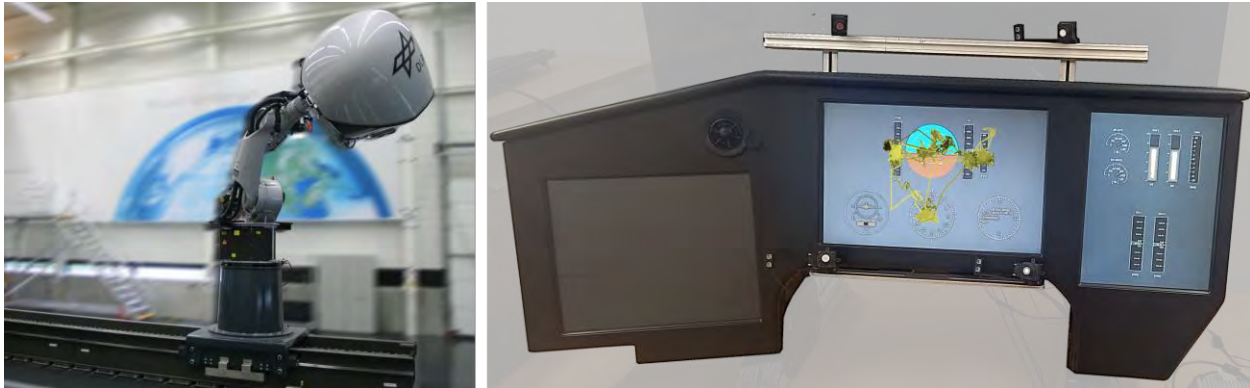
Figure 1. Left. DLR Robotic Motion Simulator (Bellmann, 2014), covering seven degrees of freedom. Right: Exemplary eye-tracking recording for standard cross check (yellow) in a generic cockpit dashboard.
