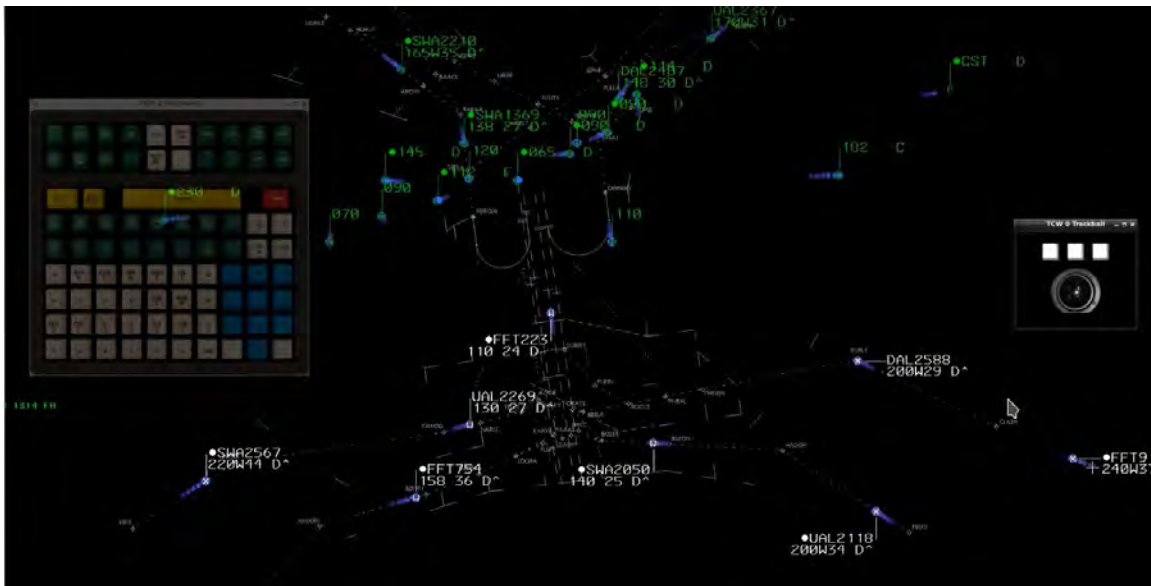
Figure 2. STARS interface showing west sector arrivals in white. Note that the trackball and keypad are virtual.
