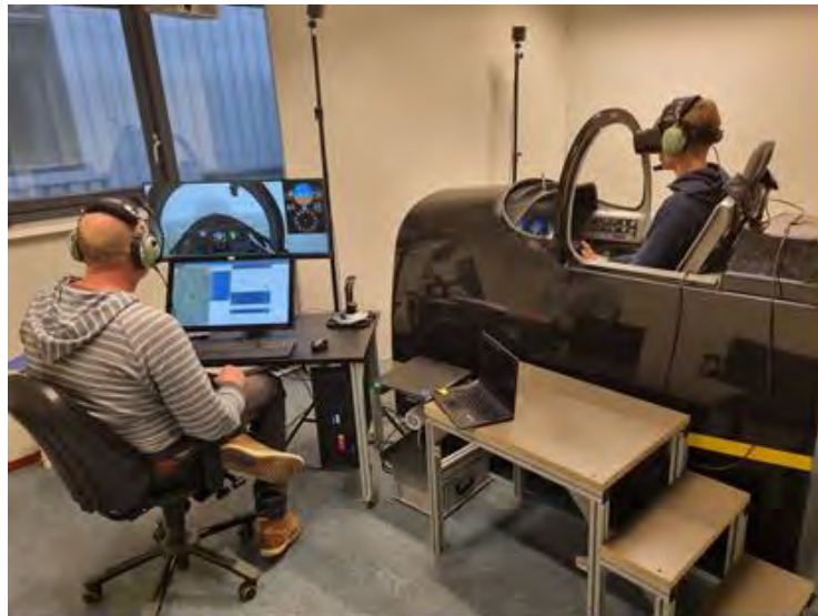
Figure 1. Setup of the VR simulator during the experiment, with the participant inside the cockpit mock-up and the experimental test leader behind the instructor station.
