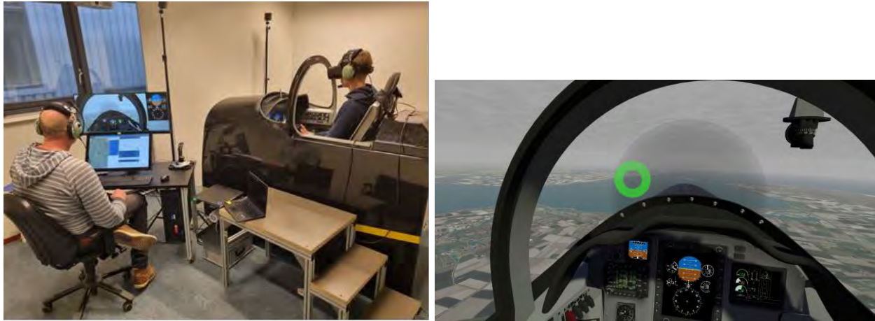
Figure 1. (A) Setup of the VR simulator during the experiment, with the experimental test leader behind the instructor station and the participant inside the cockpit mock-up. (B) Pilot view with gaze direction overlaid in green. Note: the gaze direction was not shown during the experiment.
