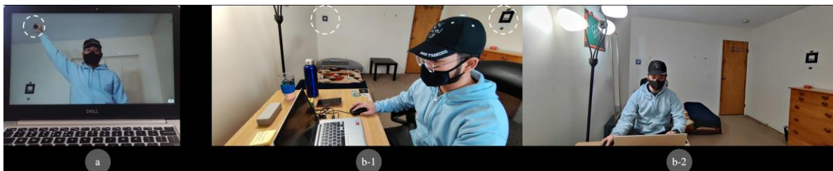
Figure 2. AR Interventions for reducing zoom fatigue (a) AR Exergame: The system detects the AR marker in the background and uses it as a reference to display 'virtual apples' (shown inside the dotted circle) in random locations. The user is required to reach out and grab the apples as they appear (b) AR Micro-movements: (b-1) The user has several AR markers in the physical working space (encircled by white circles). To enter a virtual class, a new/different marker is required to be visible in the background. To enter the next virtual class, the user is required to move to a different location such as the other side of the table so that a different unique marker is visible. (b-2) The user has physically moved to different location to enter the next virtual class.
