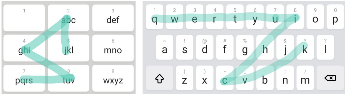
Figure 1. If the users want to type a word "QUICK" with gestures, the gesture path on the Qwerty keyboard is much more ambiguous than on the T9 keyboard.
