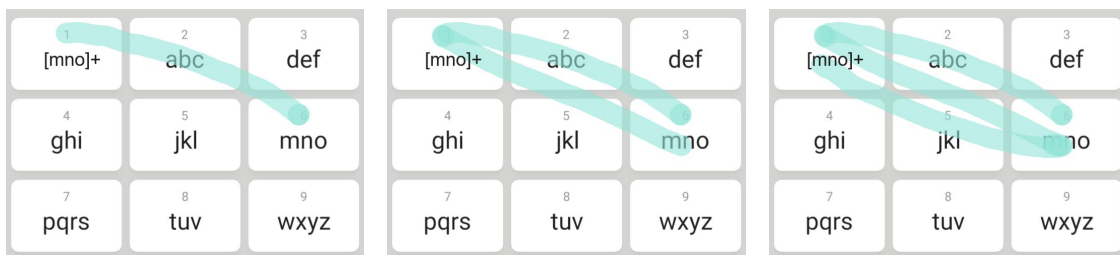
Figure 4. For inputting the word "MOON", the swipe gesture is supposed to start from key 6 to key 1 then to key 6, finally to key 1.
