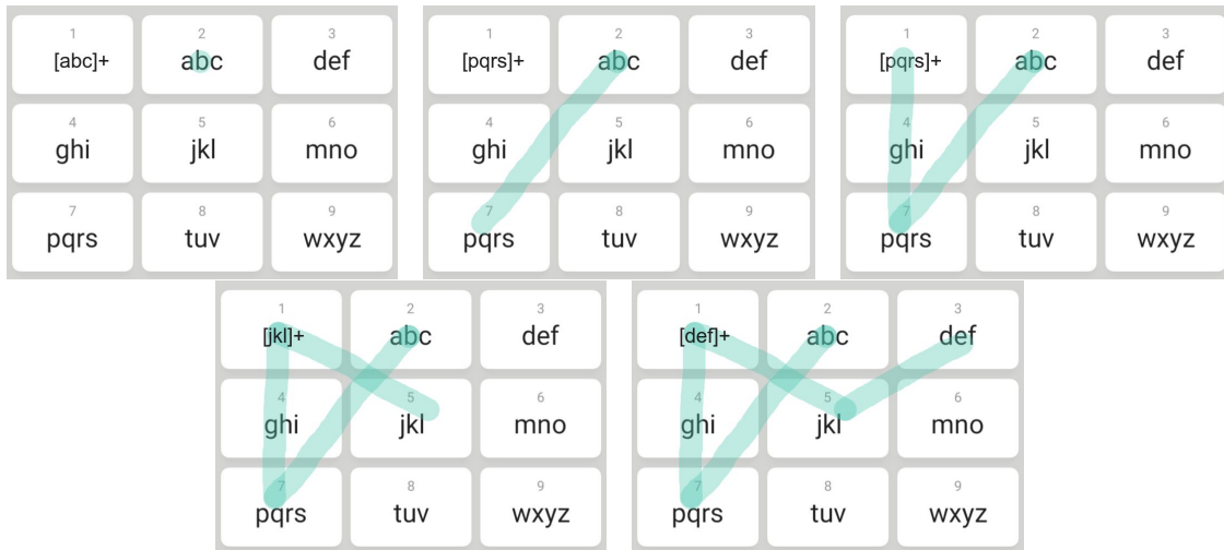
Figure 3. For inputting the word "APPLE", the swipe gesture is supposed to start from key 2 to key 7 then to key 1, finally to key 5 and key 3. The letters corresponding to Key 1 change with the movement of the finger.
