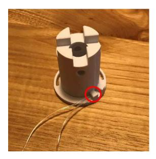
There are two rotation stop nubs on the hidden face of the modular connector. One of these rotation stops has two holes present. Insert the 6 inch length of elastic cord into the hole closest to the internal cylinder and route the cord through the second hole in the same rotation stop. The ends of the cord should come out of the nub as shown above. Make sure the free ends of the cord exit the side of the nub facing away from the second rotation stop.
