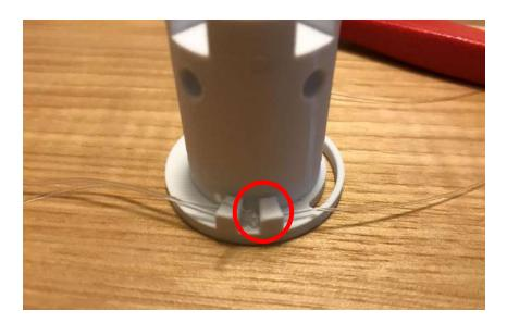
Run the length of fishing line through the remaining rotation stop nub and knot it tightly as show. The knot should be able to sit in the space between the nubs. Snip the extra length of the knot, being sure to snip enough where it will fit into the space but not too much where the knot will become undone.
