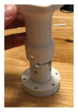
Assembly the hand receptor and modular connector by aligning the holes and pressing the two parts together. Insert the wrist pin into the hole in the hand receptor to lock the two parts together. The assembly is now complete. The fishing line will still have a free end after this assembly, the line gets routed through the forearm cup printed part.
