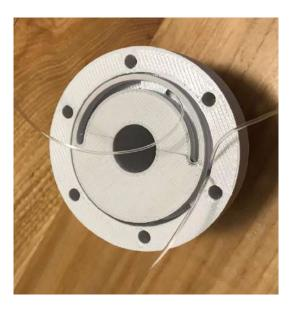
Route the fishing line through the semi-circular slot in the modular connector. Keep the ends of the elastic cord accessible. Knot the two ends of the elastic cord together, making sure to pull the knot tight to seat it in the encasement. A square knot works well here.
