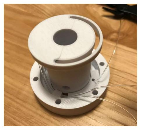
Match up the holes on the modular connector with the holes on the encasement to ensure they don't entangle. This is easiest if you place the parts together as shown above.
