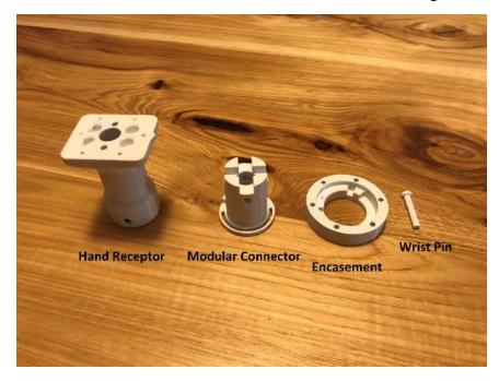
The parts picture above are the 3D printed components of the design, each is labeled with the part name. They will be referred to by these names in the assembly process.
