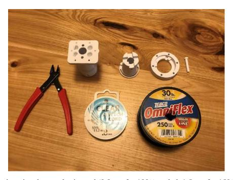
In addition to the printed parts elastic cord (0.8mm for 100% scaled, 1.5mm for 150% scale)  $30 \, \text{lb} - 50 \, \text{lb}$  fishing line is needed for assembly too, the same as that used in the assembly of the rest of the RIT Arm V2. A pair of wire cutters and thin needle nose pliers (not pictured) are recommended tools. About 6 inches of elastic cord and 48 inches of fishing line will be used.
