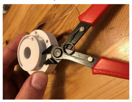
Cut the ends of the elastic cord quite close to the knot, while keeping some space to keep the cord secure.
