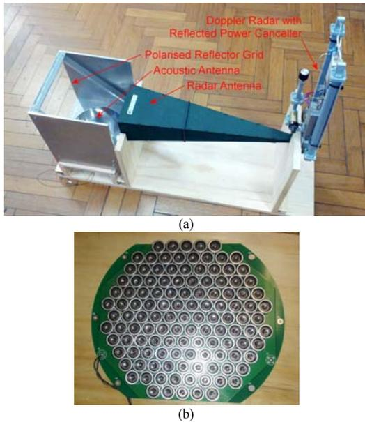
Figure 3. Photograph (a) of the mesh reflector based RASS and (b) a the 131 element sonar array
