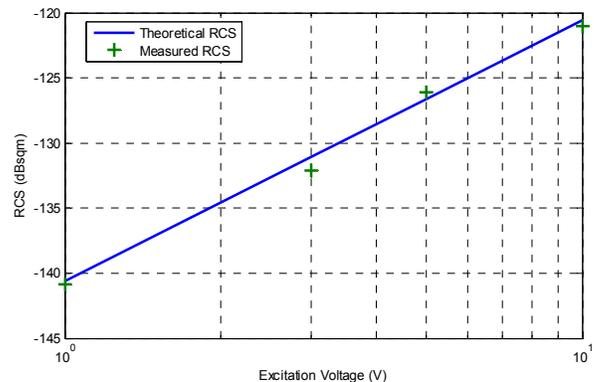
Figure 6. Mean Doppler target RCS at different peak to peak excitation voltages compared to the simulated RCS at the same excitation voltage
