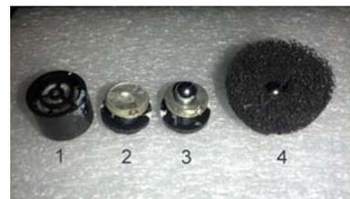
Figure 5. Construction of a small Doppler target from a piezo transducer and a small ball bearing
