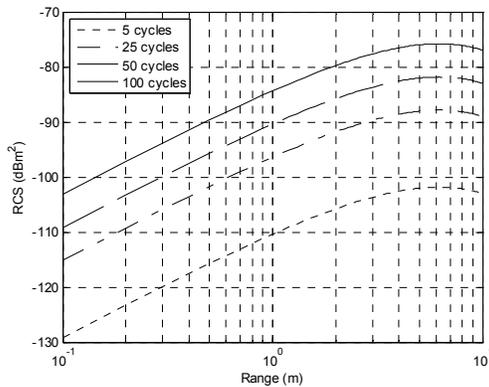
Figure 4. Radar cross section of an acoustic pulse with the number of cycles,  $N$ , in a pulse as a parameter
