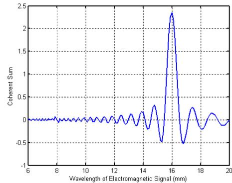
Figure 1. Coherent sum of the reflected signals shows the Bragg Condition
