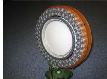
Figure 2. Monostatic RASS configuration using a central horn lens antenna surrounded by a double ring of small ultrasound transducers
