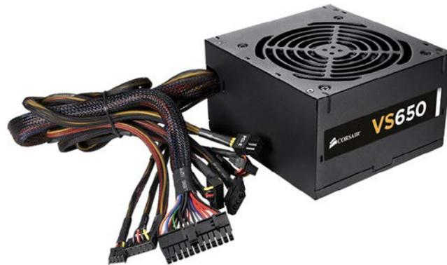
Find the connectors which plug into the Hard Drive (if needed), GPU (if needed) and the Motherboard, then connect them.
