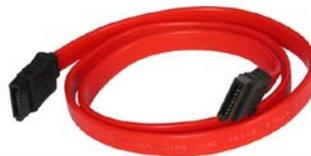
Connect one end to the Hard Drive or SSD and the other to the Motherboard
