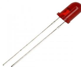
This is what we will use to see if the circuit operates correctly. Attach the LED somewhere in the horizontal batch of holes. Location doesn't matter, but the shorter wire is the negative side, and the longer is the positive. If put in the wrong direction, the LED won't light!
