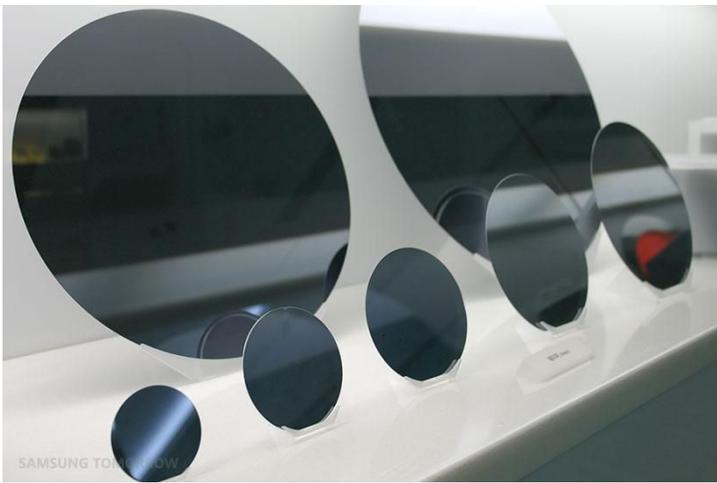
**Silicon Wafers Before Processing**
