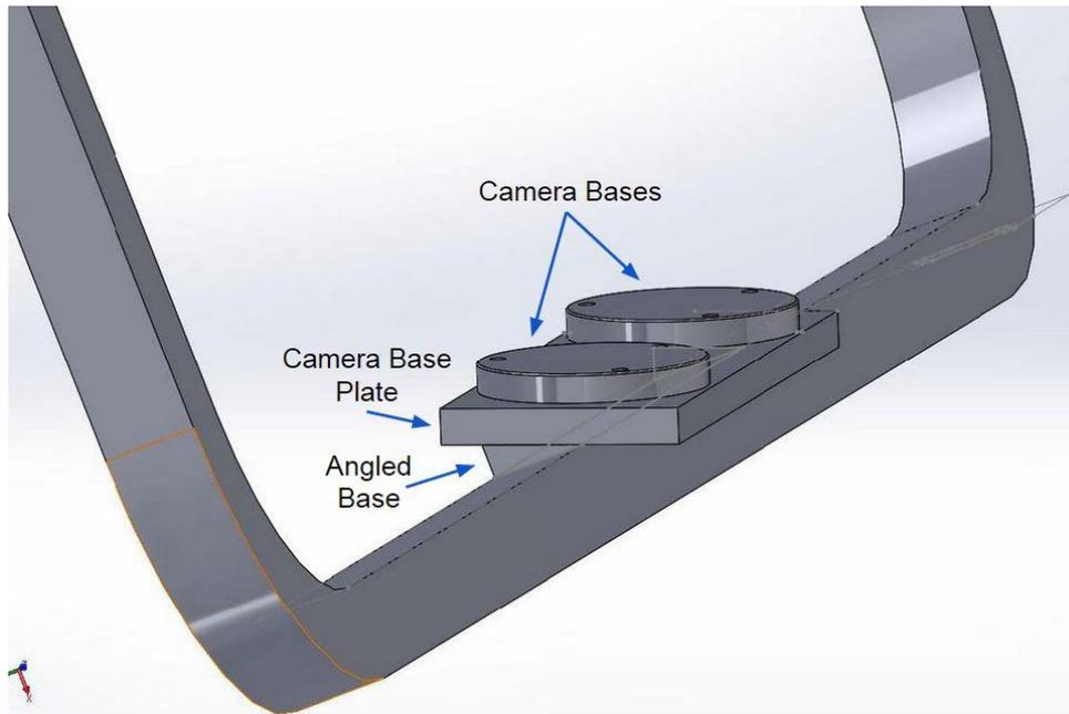
**Figure 9: Stereo Camera Mount**
