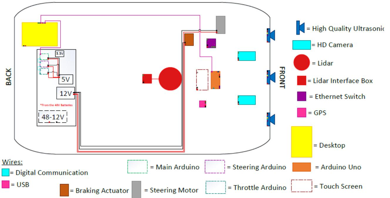
Figure 6: Phase I & II Overlay Wiring Layout
