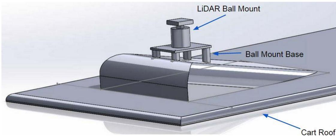
Figure 7: Preliminary LiDAR Mount
