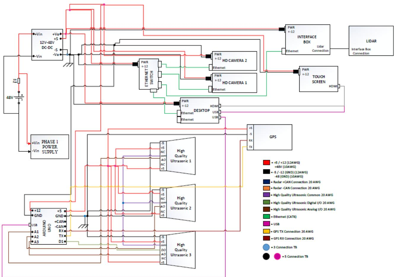
Figure 3: Phase II Overall Wiring Diagram
