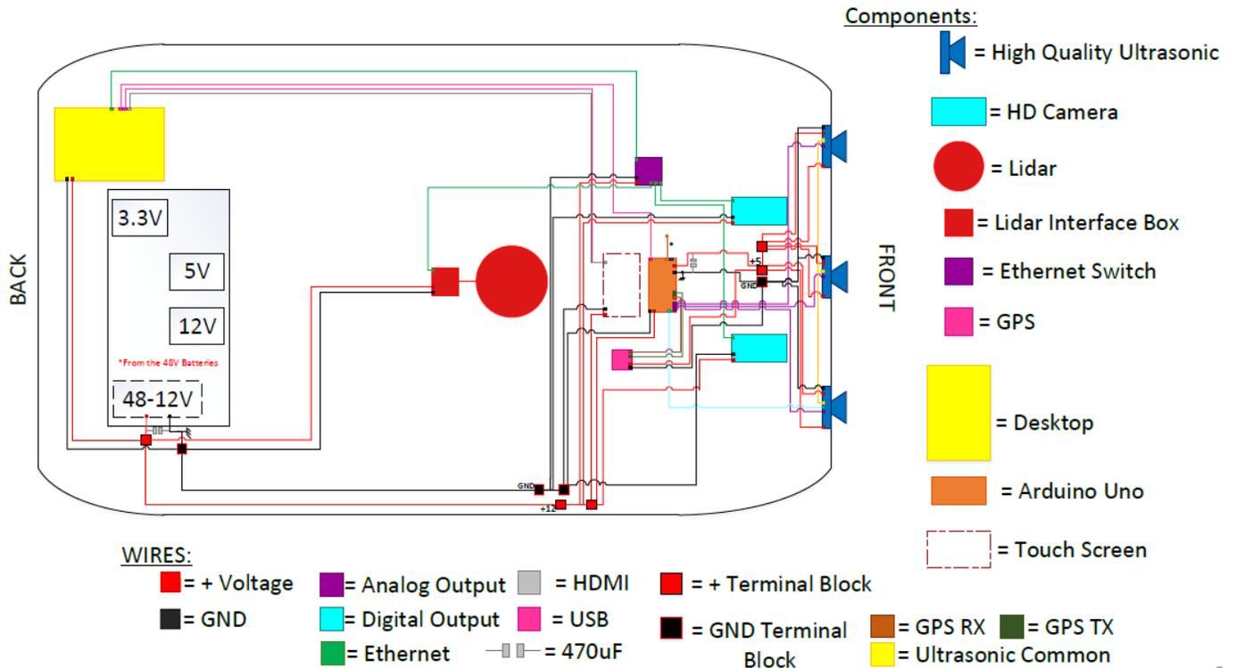
Figure 5: Phase II Overall Wiring Layout
