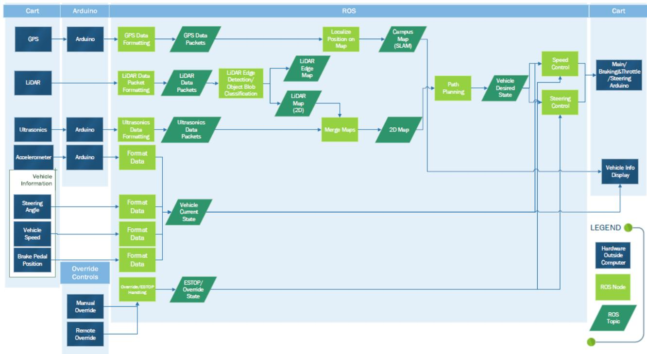
Figure 1: Complete People Mover Software System Flow Diagram
