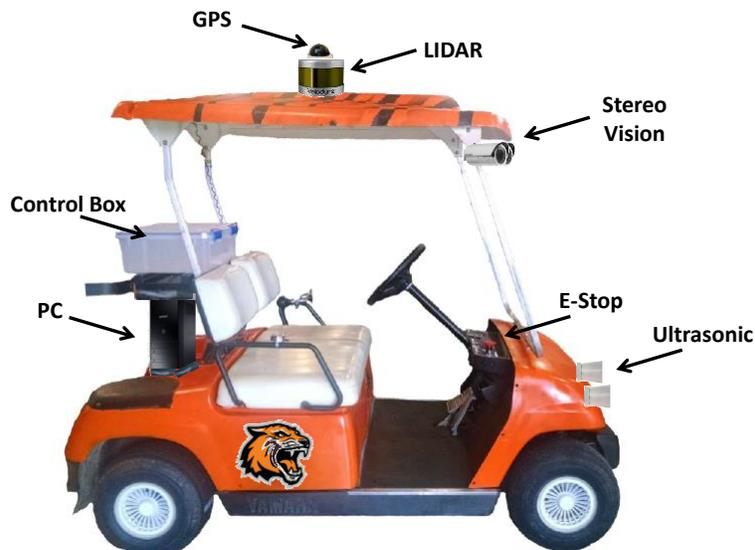
Figure 4: Sensor Placement on Cart
