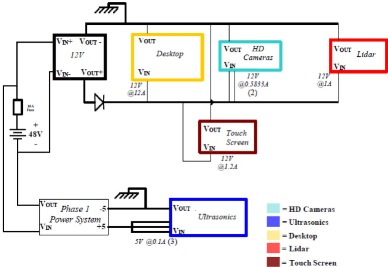
Figure 2: Phase II Overall Power Diagram
