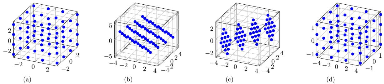
Fig. 4: An illustration of the number of dimensions available in the wireless channel. In (a), each blue dot represents a 3-D signal. This set of signals is pre-rotated before transmission (b). The channel rotates and scales the signals (c), which are finally post-rotated at the receiver. This shows that the channel may transmit signals in three dimensions.
