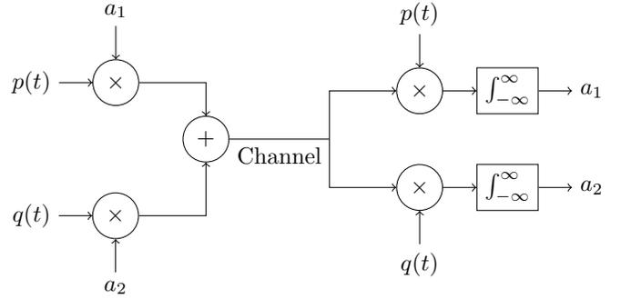
Fig. 1: Transmission of two numbers,  $a_1$  and  $a_2$ , using orthonormal signals  $p(t)$  and  $q(t)$ . The channel is an electronic medium. In the absence of noise, the numbers are recovered perfectly by the receiver.
