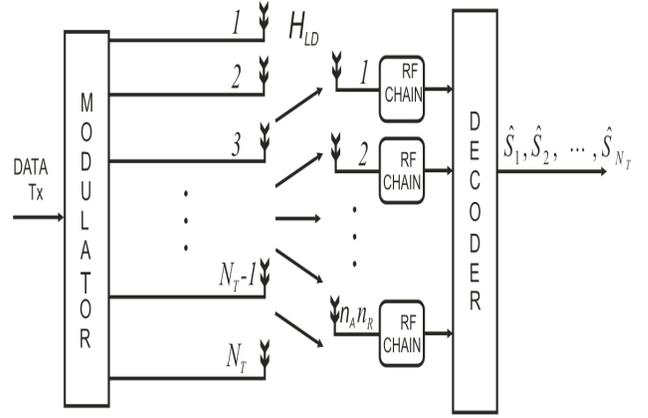
Fig. 6: A hybrid system equivalent to that of Figure 5, once it has been converted to a linear dispersion code. This conversion means that all known results for spatial-multiplexing codes are immediately applicable to this hybrid code.
