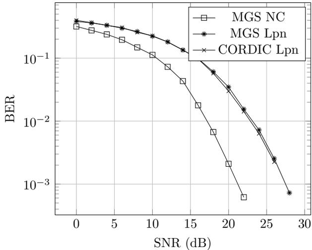
Fig. 11: Hybrid code performance loss when the channel presents Laplacian correlation. Under this channel, the CORDIC requires 8 iterations to reach the performance predicted by the modified Gram-Schmidt algorithm.
