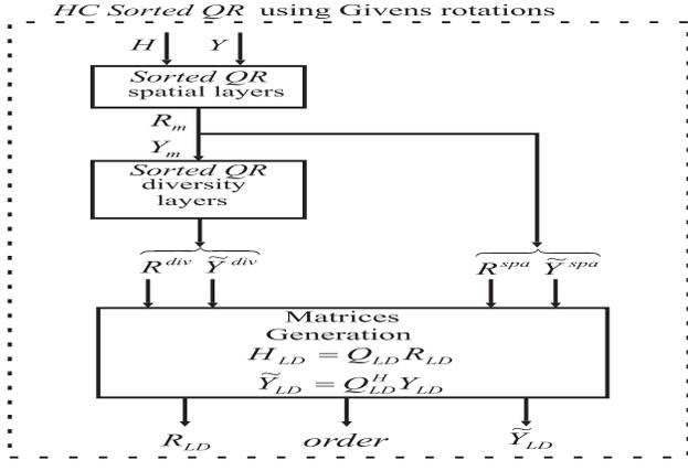
Fig. 7: Detection process for hybrid codes. Using Givens rotations, this process may be implemented in hardware with low complexity.
