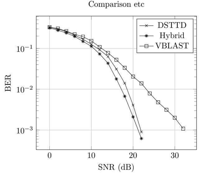
Fig. 9: Bit-error rate comparison between DSTTD, hybrid, and V-BLAST space-time codes. The hybrid code described here is the better performer.
