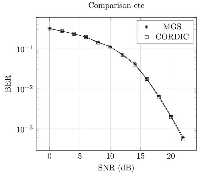
Fig. 10: A comparison between code performance when the QR decomposition in the receiver is performed using the modified Gram-Schmidt algorithm or with CORDIC. Here, the CORDIC performs seven rotations, which are enough to reach the best performance.
