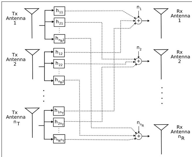
Fig. 2: A system with multiple transmit and receive antennas. The signal between each pair of antennas is multiplied by the channel gain, which changes the signal's amplitude and phase. Each antenna receives also a noise signal. All channel gains and noise signals are independent of each other.
