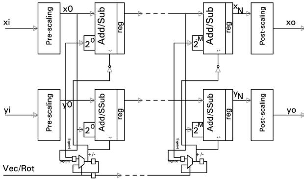
Fig. 8: Diagram of a CORDIC processor.
