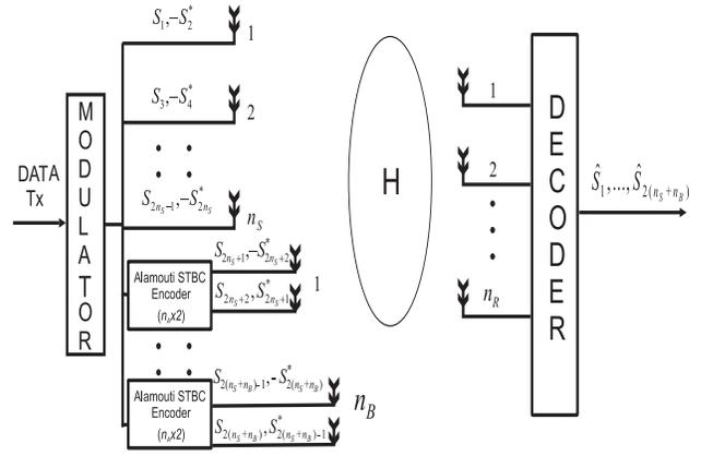
Fig. 5: Block diagram of the ZF LD STBC-VBLAST hybrid code. The code consists of  $n_S$  spatial layers and  $n_B$  diversity layers.
