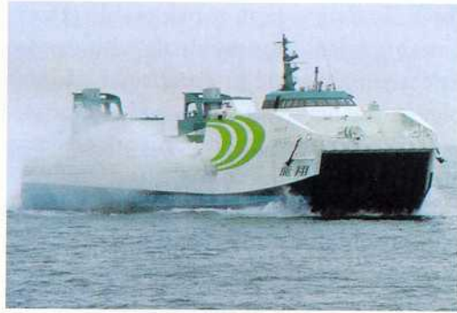
Our support has enabled the development of exciting new technologies such as this Techno-Superliner, which is capable of transporting freight at speeds of up to fifty knots.
