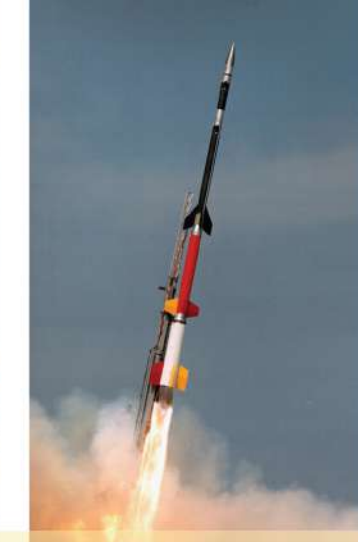
ABOVE: The CIBER-2 mission will be launched on a Black Brant sounding rocket similar to this one, seen launching from NASA's Wallops Flight Facility in Virginia. NASA
