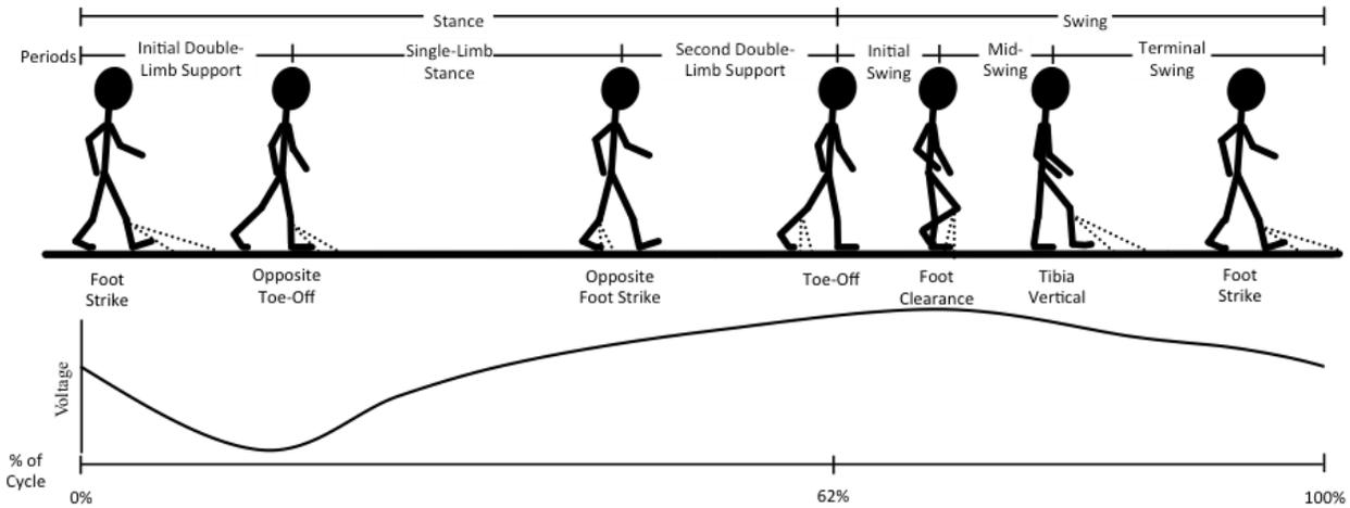
The sensors work by looking out ahead of the user and measuring the distance to the upcoming terrain. A representative sensor profile is shown here, corresponding to a pattern of level walking.
