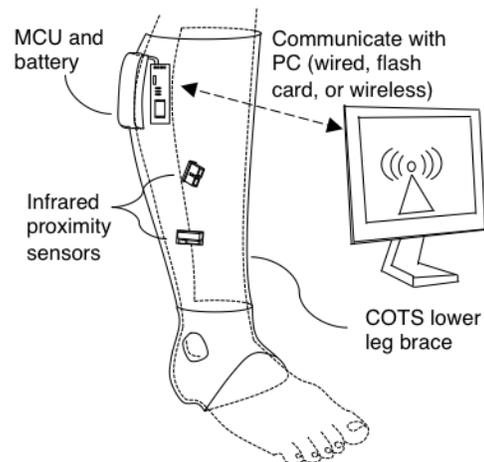
The system is comprised primarily of commercial, off-the-shelf parts and can be easily attached to the leg.
