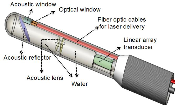
Figure 1: Photoacoustic Prostate Probe
