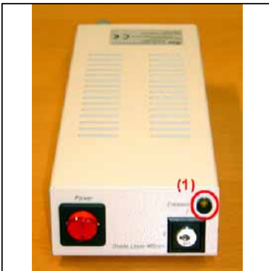
figure10. Emission warning indicator of the external 405-nm Advance laser
