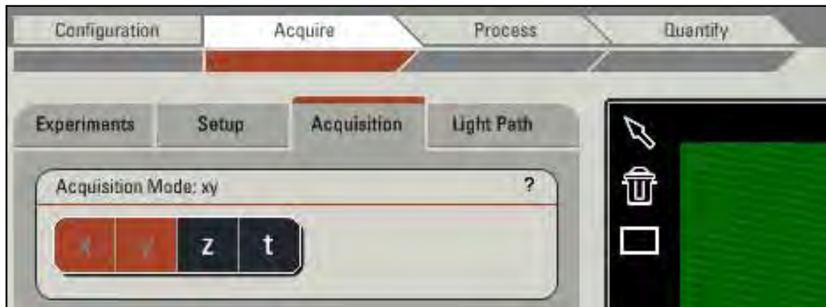
figure51. Use the "Acquire" arrow button to acquire data in all Leica LAS AF applications.
