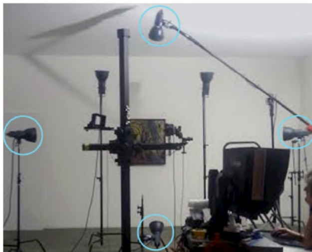
Figure 1. Lighting setup using four different strobes for illuminating objects from four different directions. The lights are positioned to the top, bottom, left and right of target area. This image was taken at the Museum of Modern Art, Queens, as part of an imaging demonstration.
