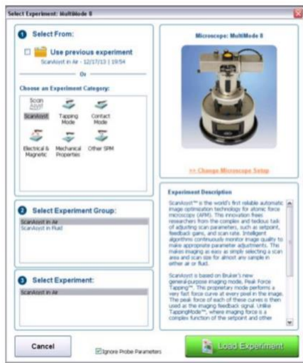
Figure 3) Experiment selection: Screenshots of experiment selection for Scanasyt. Tip , use USER experiment if unsure what to use, or contact POC.
