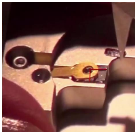
Figure 2) Tip holder assemblies for a solid-state sample.
