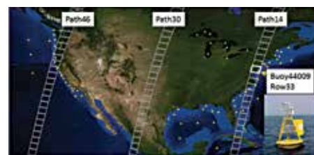
Figure DIRS5: Array of buoys used for thermal calibration of Landsat
