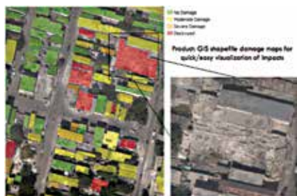
Figure DIRS13. Examples of disaster response products that Colin Axel (PhD student) is developing using the fusion of high spatial resolution color imagery and discrete lidar sensing. (Top) A building damage assessment map, developed using lidar metrics
