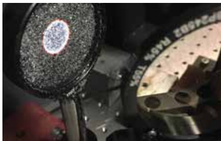
Researchers made a mirror surface out of glitter to test the idea of using a cloud of reflective particles as a space telescope mirror. They took images of two light sources using this mirror in a laboratory at Rochester Institute of Technology. Credit: G. Swartzlander/Rochester Institute of Technology.
