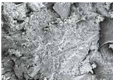
Fig.9. SEM images of the cement material after curing. Left, control, right, improved version with higher compressive strength by omitting one of the raw materials.
