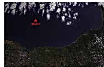
Figure DIRS6. An example of a Landsat image of Lake Ontario with a buoy in the scene (the red triangle indicates the buoy location). The temperature at the buoy location is estimated using the LST process and is compared to the buoy measurement that was taken at the time of acquisition.
