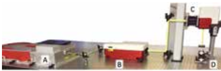
Fig. 1. Femtosecond laser processing system at RIT/AOFIM lab: (A) Femtosecond laser (Amplitude), (B) beam modification device (LASEA), (C) 3-axis optical beam scanner, (D) 3-axis sample positioning stage.
