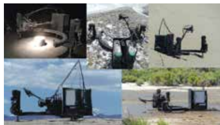
Figure DIRS-4. Images of the new GRIT-T deployed in different scenarios. Clockwise from upper left: Laboratory setting with artificial illumination on an engineered sediment, view showing the dual spectrometers used by the system, leveled instrument on a steep dune slope, use on a coastal tidally flooded site, and detail of the leveling legs and articulated probe.
