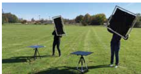
Figure DIRS-3. Left. The use of shadowing on grayscale calibration targets to provide a means of image calibration for improved calculation of normalized difference vegetation index (NDVI) in shadowed conditions by tall trees or buildings or by clouds. This type of calibration adjustment is necessary to fully exploit the ability of a UAS to fly and collect calibrated data under varying atmospheric conditions such as under clouds.
