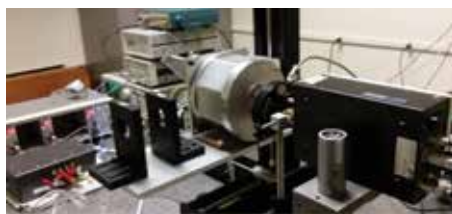
Figure 7: A photo of experimental setup is shown above. The source is on the right, followed by the shutter, and the test dewar enclosure. The enclosure is mounted on XYZ and rotation stages for alignment of the MOSFET of interest with the source. Response is viewed in real-time for alignment with a source measurement instrument, or a lock-in.
