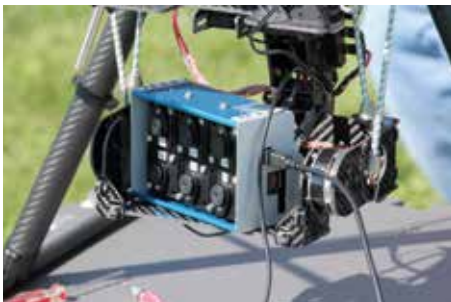
Figure DIRS-2. A 6-band multispectral Tetracam, Inc. camera system installed on a gimbal hanging from an octocopter. The use of red and near infrared filters on two of the cameras allows the calculation of NDVI.
