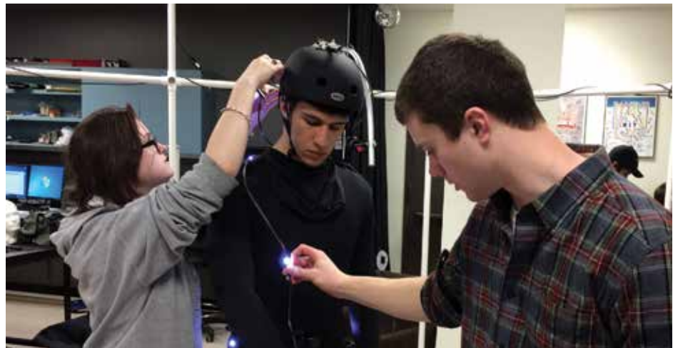
Freshmen Ari Porkos and Lenny Wilkinson make adjustments to light emitting diodes on a student-developed motion capture suit being worn by Peter Jarvis.
