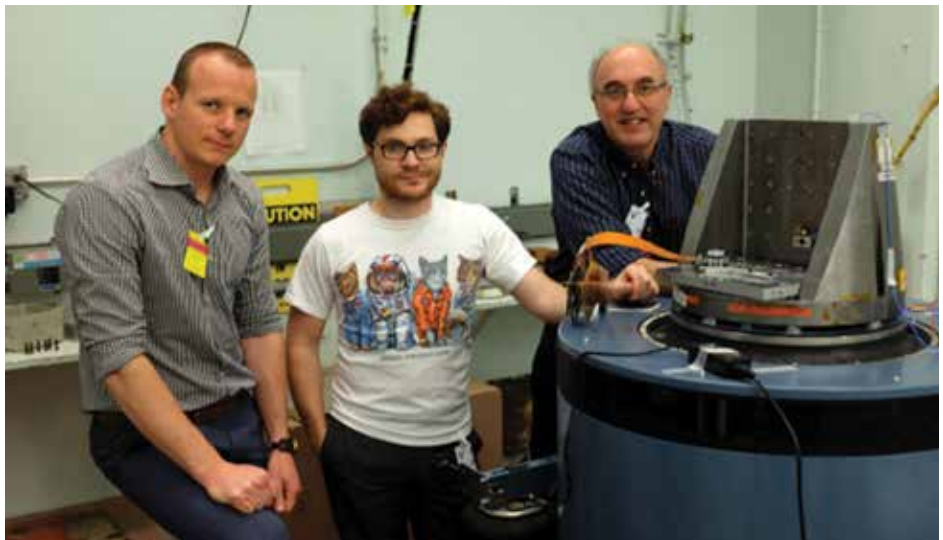
Figure 2: Travinsky, Vorobiev and Ninkov next to the shake table at NASA GSFC. The DMDs under test are mounted in a plate on the shake table and the interface cable is seen going to the control board.
