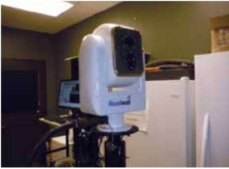
Hyperspec and Hyperspec_closeup. (Left) New hyperspectral imaging system during a test on the RIT campus in June 2017. The system incorporates a Headwall micro Hyperspec high-efficiency mounted on a General Dynamics Maritime pan-tilt and deployed on a telescopic mast. (Right) Close-up of the integrated Headwall Hyperspec and General Dynamics pan-tilt mount in Dr. Bachmann's GRIT Laboratory.
