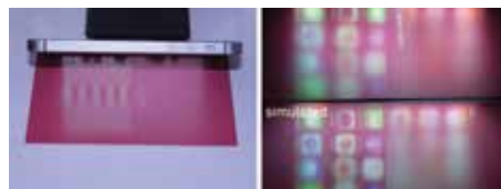
Figure 1: (left) Grating image on smartphone reflected in sample surface to estimate surface roughness. (right) Smartphone image reflected in real surface (top) and simulated surface (bottom) estimated using the method.
