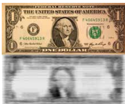
Figure 1. Images of the optical (top) and magnetic (bottom) inks on a US one dollar bill. Bottom image was recorded by rastering the bill over the surface of the EPR MOUSE.
