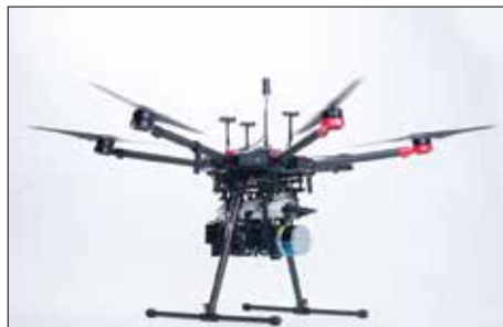
Figure MX1. MX1 payload incorporating hyperspectral, lidar, thermal infrared, and color visible sensors onto a single platform.
