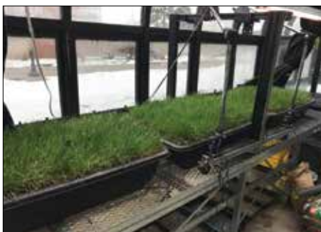
Figure Methane. Experiment to investigate observable effects on healthy vegetation stressed by methane leaked into soil.
