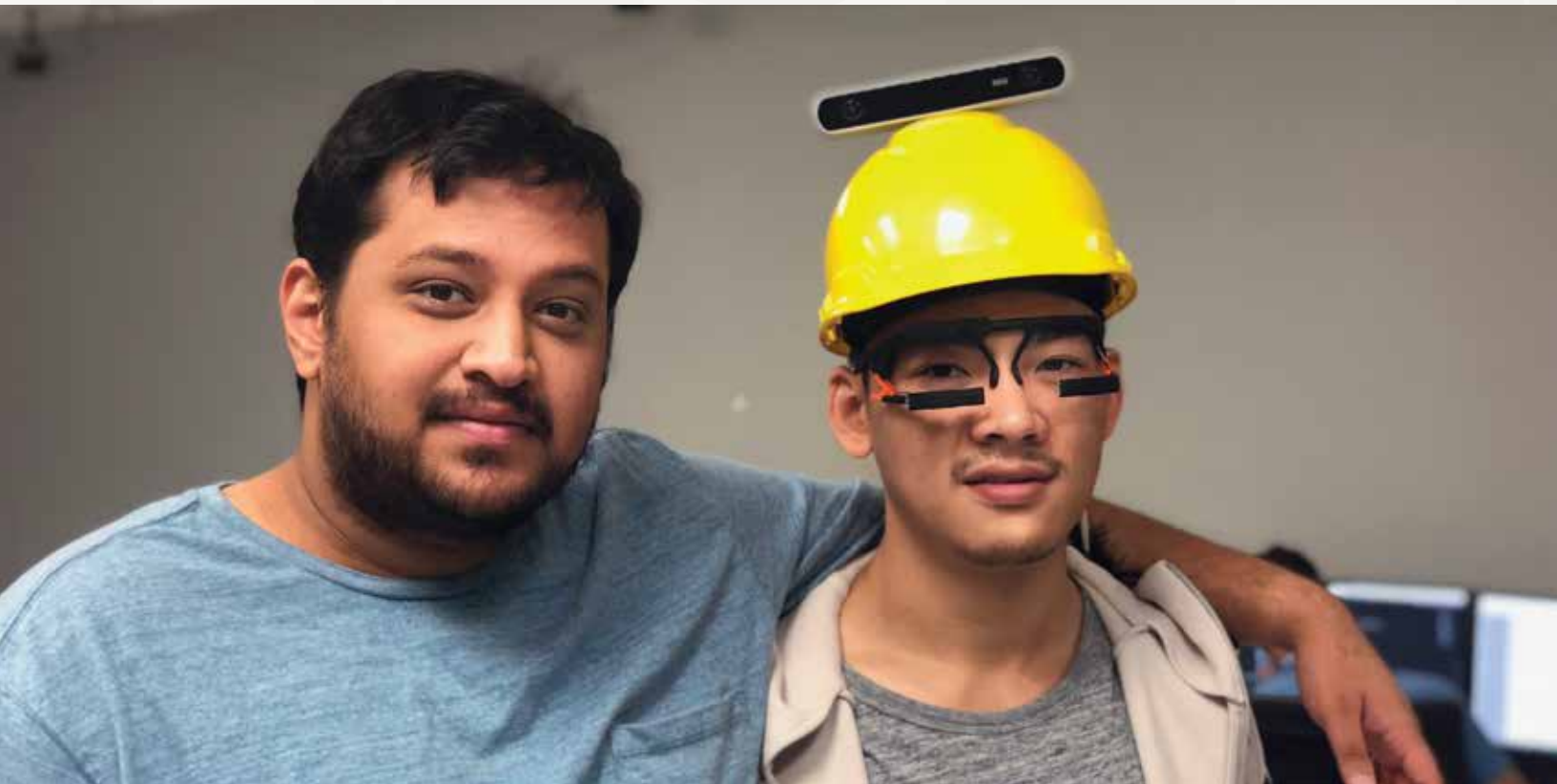
Rakshit Kothari (left) poses with Zhizhuo (George) Yang (right), who is wearing a custom-made system for the collection of eye + head pose when performing natural task. This involves record movements of the eyes with a Pupil Labs mobile eye tracker, and the head with an internal measurement unit, and the scene color and depth maps with stereo RGB cameras. This system is being used for the development of novel machine learning algorithms for understanding the gaze behavior of observers during navigation and task execution.
