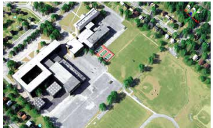
Hyperspectral (i.e., 500 to 2500 nm) DIRSIG rendering (w/o sensor PSF) of Megascene 1 with RGB bands overlayed onto a DIRSIG generated 3D LiDAR image. Notice T-72 tank targets placed in the open, along a tree-line, and next to a building (Gartley et. al.).
