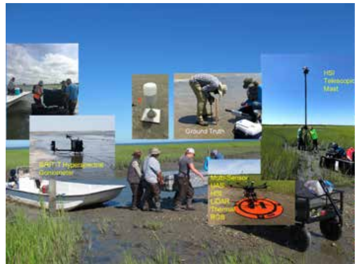
Figure 1. Field validation of models for retrieval of sediment geophysical properties using multi-temporal and multi-view have been the core of our project. Inset photos show (right) the hyperspectral video imaging system deployed on a telescopic mast, (middle) one of the UAS systems with a multi-sensor payload including hyperspectral, LiDAR, thermal, and framing RGB imaging systems as well as ground truth data collection in the field, and (left) our hyperspectral Goniometer of the Rochester Institute of Technology – Two (GRIT-T), which measures the directional dependence of spectral reflectance in both field and laboratory settings.
