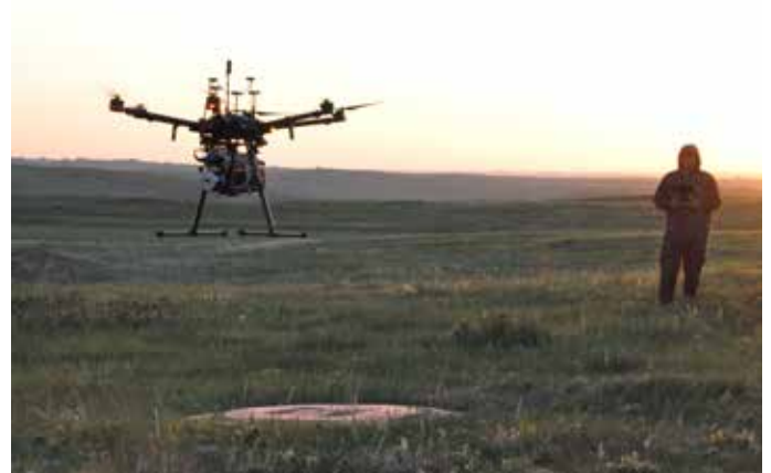
Figure 2. UAS pilot Tim Bauch collecting early-morning thermal imagery on the prairies of North Dakota for duck nest detection
