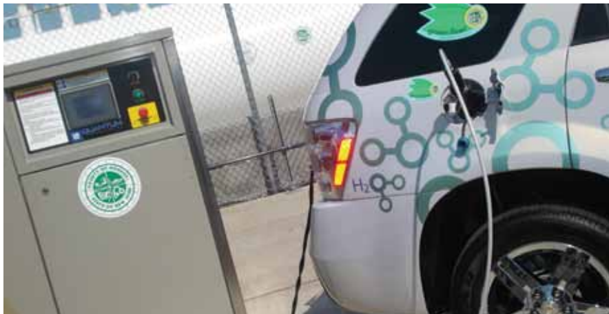
Alternative Fuels: An alternative fuel test vehicle being filled with hydrogen at a county refueling station. Golisano Institute researchers are currently testing the performance of hydrogen vehicles in partnership with General Motors.
