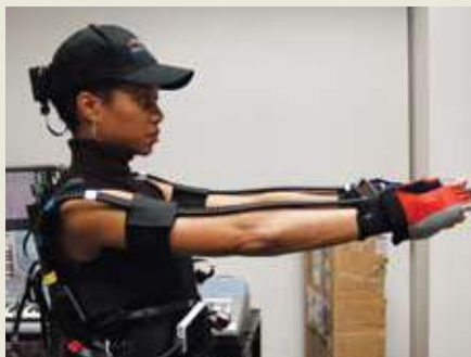
Human Performance and Internet Avatar - Tina Chapman DaCosta wears a full body motion capture suit preparing to control the motions of an avatar on the virtual stage. The avatar in the computer image follows her motion in the performance.
