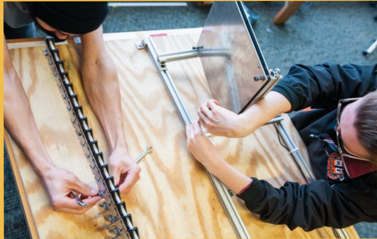
Students Joseph Samuelson, left, and Ryan Kent adjust the model tail and the electronic sensor pad to assess the impact of the tail as it moves.
