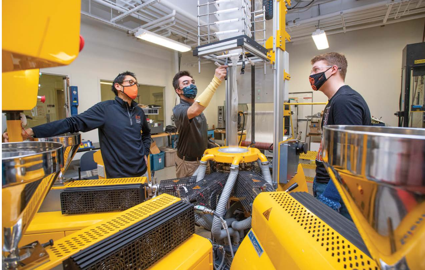
RIT professor Changfeng Ge, left, and packaging science majors Andrew Morris and Nathanael Strong research recycled plastics using the Lab Scale Blown Film Line in the American Packaging Corp. Center for Packaging Innovation on campus.
