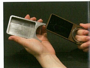
A cell phone designed by a team of RIT industrial design students can be easily disassembled, allowing components to be replaced.
