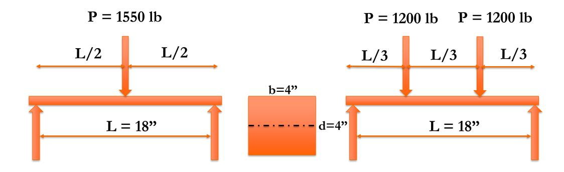
Goal-Determine the bending stresses in the two concrete beams shown above?
