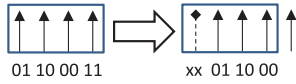
Fig. 8. Example of the FO attack on four subcarriers (left): The attack shifts the subcarriers and the corresponding bits to the right.
