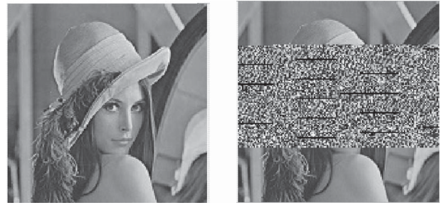
Fig. 15. Applying the FO attack on a sequence of frames belonging to an image.
