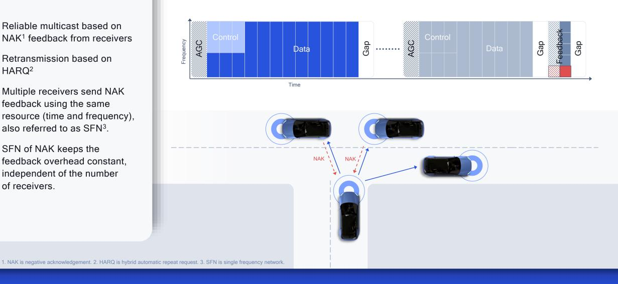
Reliable and efficient multicast using SFN feedback
