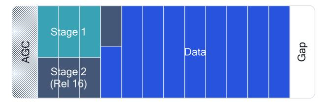
Slot structure showing two-stage control
