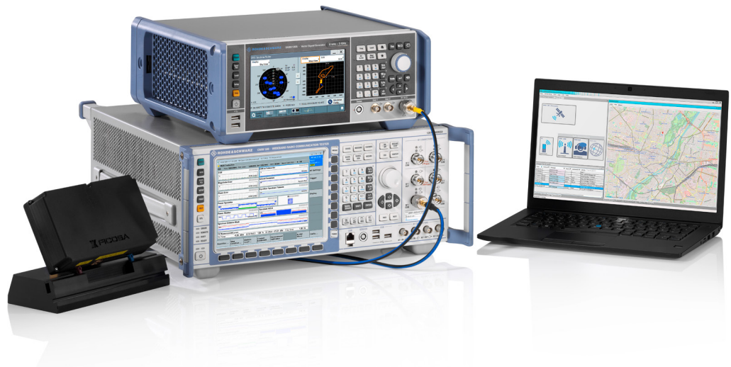
Fig. 70: eCall and NGeCall test setup
