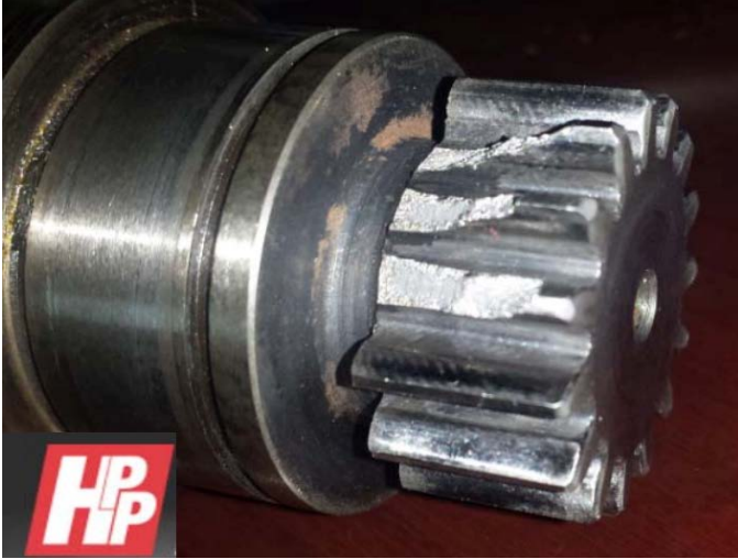
Broken teeth on the machine's drive gear; a total of five (5) teeth were damaged after more than 50 years of use.
