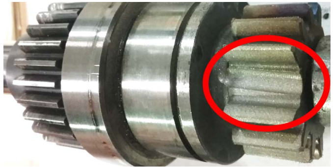
Preparations for LENS repair required machining away the old teeth
