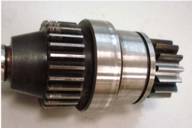
Full photo of final form achieved by machine finishing at Hansford.
