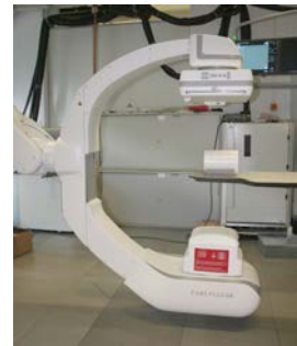
Fig. 4: Experimental set up with C-arm system and calibration phantom
