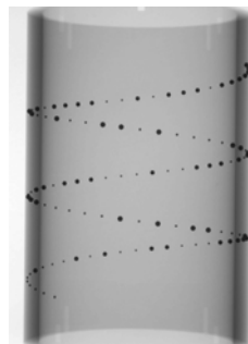
Fig. 3: Example X-ray image of the helical calibration phantom
