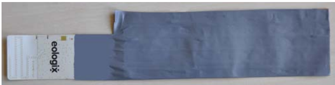
Fig. 4. Capacitive proximity sensor 270 mm \times 60 mm in size, where the gray area is the isolation layer of the electrodes.
