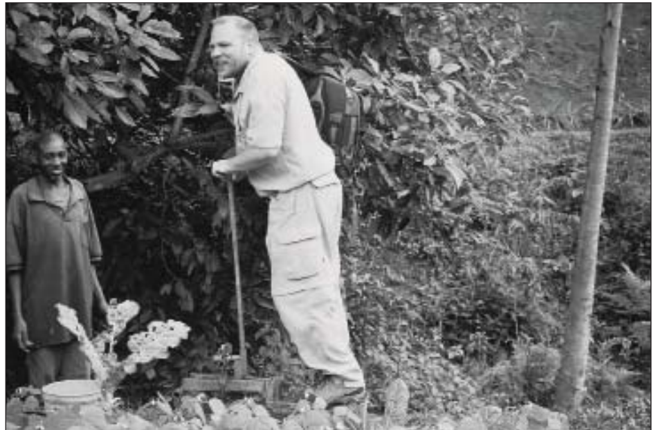
Kenneth Weimar '90, demonstrates a manual irrigation pump to a farmer in Kenya.
